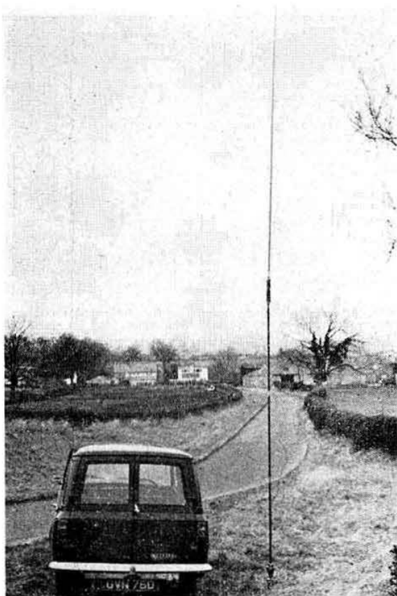
The 22ft loaded vertical is self-supporting at normal wind speeds. Guys may be added during gales
